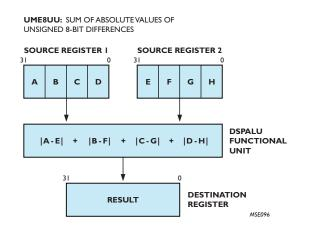
The PNX1500 CPU's special 'ops' dramatically improve performance and increase the efficiency of its parallel architecture. The ume8uu operation, commonly used for motion estimation in video compression, implements 11 simple operations in one TriMedia special op.
